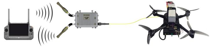
This type of architecture is used for either commercial hazardous area inspection or for military target strikes. The fiber can be either a fixed hybrid cable for stationary applications or up to 40km long for military strikes.
