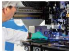
Ray Photonics' automatic wire bonder
